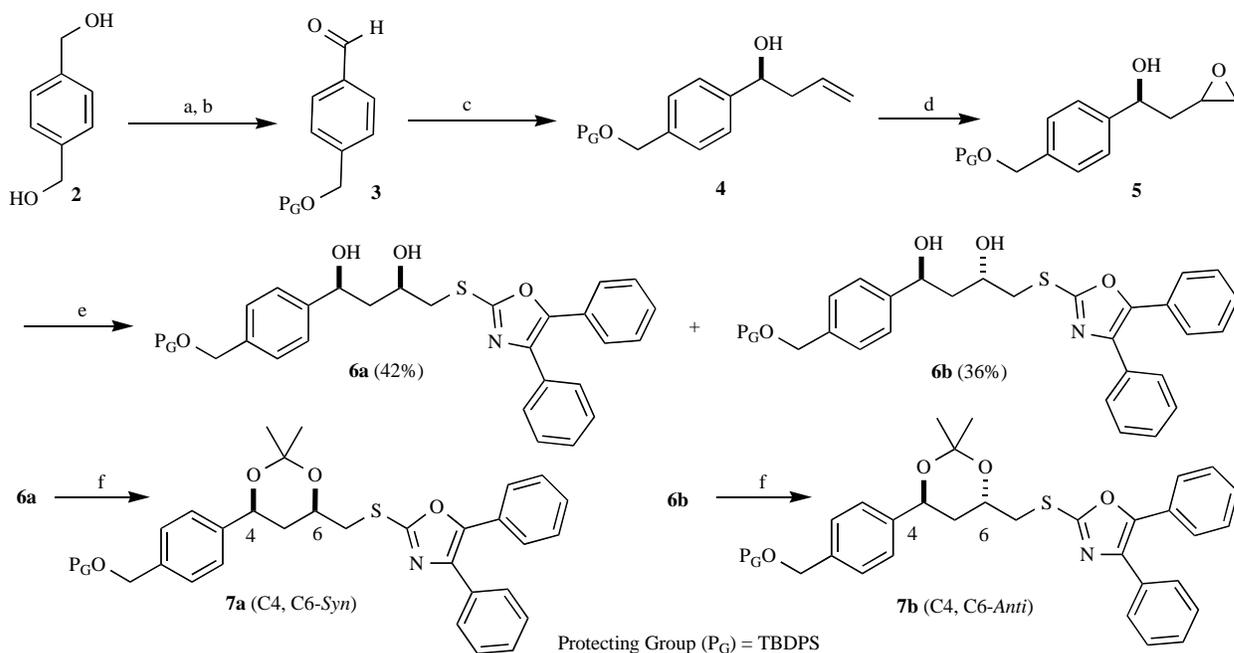
**Scheme 1.** Reagents and conditions: (a) TBDPSCl, imidazole, DMF, 50 °C, 16 h, 42%; (b) MnO<sub>2</sub>, CH<sub>2</sub>Cl<sub>2</sub>, rt, 12 h, 92%; (c) (-)-Ipc<sub>2</sub>BAl, Dioxane, Et<sub>2</sub>O, -100 °C, 2 h, 65%; (d) *m*-CPBA, CHCl<sub>3</sub>, rt, 24 h, 75%; (e) 4,5-diphenyloxazole-2(3H)-thione, DIEA, DMF, rt, 78%; (f) Me<sub>2</sub>C(OMe)<sub>2</sub>, TsOH, rt, 12 h, 76-80%.
