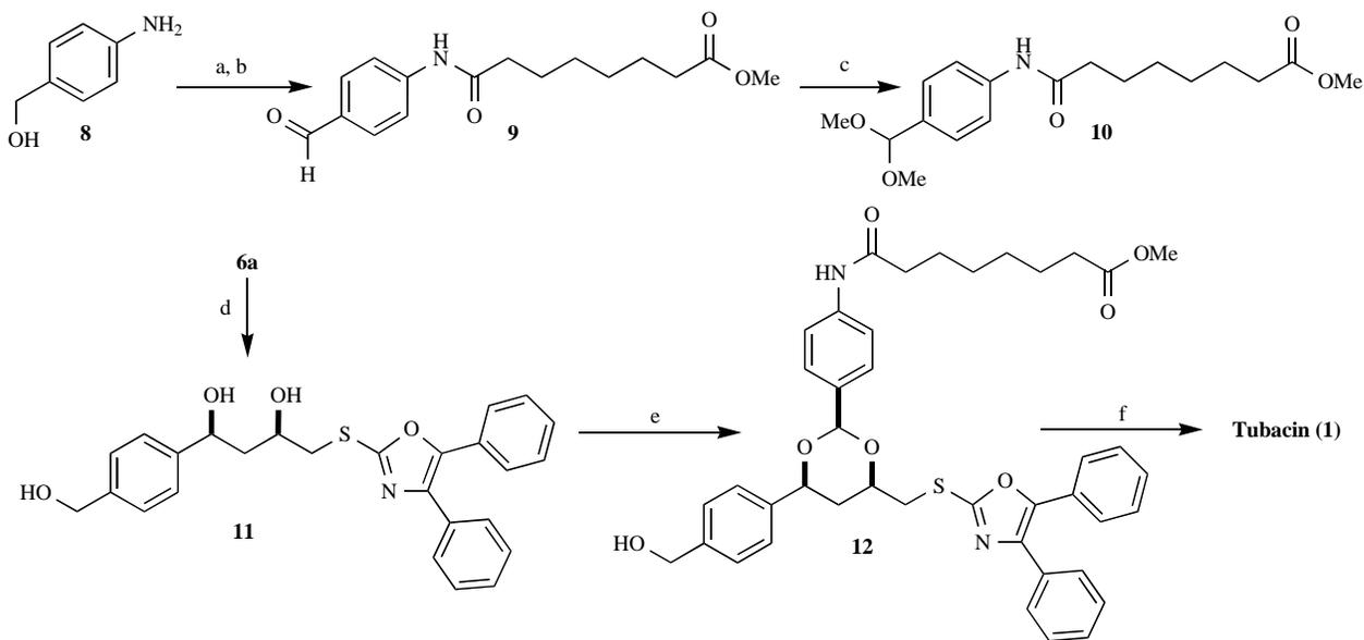
**Scheme 2.** Reagents and conditions: (a) Methyl 8-chloro-8-oxooctanoate, Et<sub>3</sub>N, CH<sub>2</sub>Cl<sub>2</sub>, rt, 10 h, 61%; (b) MnO<sub>2</sub>, CH<sub>2</sub>Cl<sub>2</sub>, rt, 16 h, 90%; (c) HC(OMe)<sub>3</sub>, TsOH, MeOH, reflux, 2 h, 94%; (d) TBAF, THF; (e) **10**, PPTS, DMF, rt, 12 h, 74%; (f) NH<sub>2</sub>OH.HCl, KOH, MeOH, rt, 46%.
