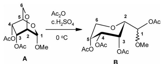
Scheme 1. Acetolysis of a 2,6-*O*-anhydropyranoside.
