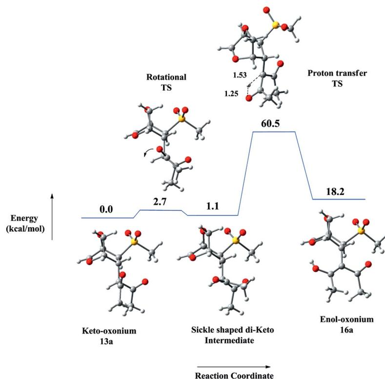
Figure 3. M06-2X/6-311+G(d)//B3LYP/6-31G(d) calculated relative energies of keto to enol transformation of the oxonium ion in TFA. All distances are in Å. Relative energies are given in kcal/mol [gray: carbon; white: hydrogen; red: oxygen; yellow: sulfur].
