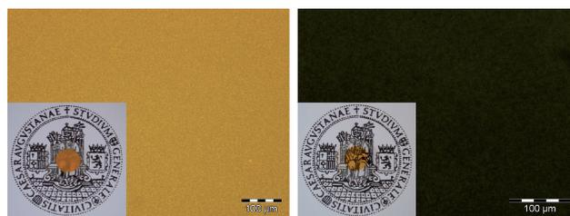
**Fig. 5** Microphotographs taken at room temperature of a sample of P8S cooled from the isotropic state at 1 °C/min (a) and 20 °C/min (b). Insets: photographs of a sample of P8S cooled at 1 °C/min (translucent sample, a) or 20 °C/min (transparent sample, b).
