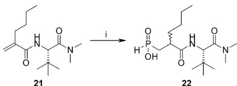
**Scheme 7.** (i) H<sub>2</sub>PO<sub>2</sub>NH<sub>4</sub>, BSTFA, 17%, then separate diastereoisomers (preparative HPLC).
