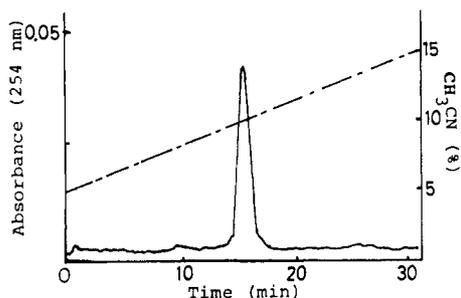
**Figure 3.** Reverse-phase HPLC of nonanucleotide on Finepak SIL  $C_{18}$  ( $4.6 \times 250$  mm). Elution performed with a linear gradient of acetonitrile (5–15%) in 0.1 M ammonium acetate (pH 7.0) in 32 min.
