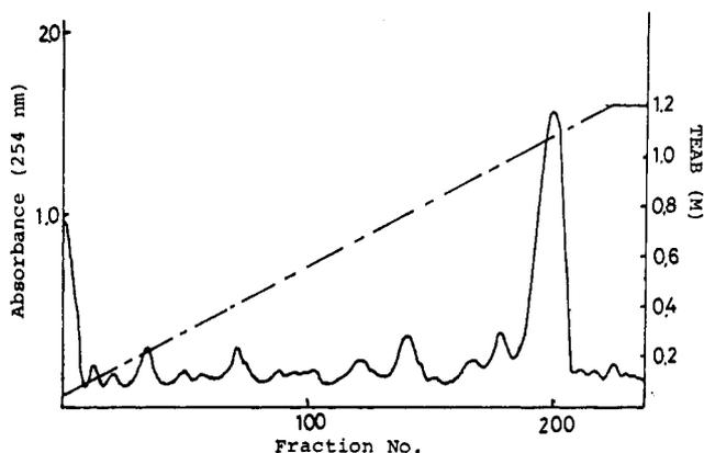
**Figure 2.** DEAE-Sephadex chromatography of the nonanucleotide. Elution was performed with a linear gradient of TEAB (0.05–1.2 M, total 1.2 L). Fractions of 5 mL were collected each 20 min. The main peak contained the product UpUp-CpApCpCpApCpA.
