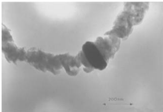
Figure 5. Typical appearance of carbon filaments produced from the decomposition of ethylene at 600 °C with Co/Ag catalyst having a high cobalt content.
