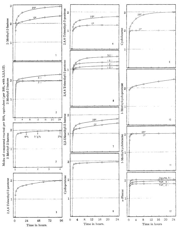
of olefin reacted per BH<sub>3</sub> were 1.35, 1.20 and 1.08 for reaction mixtures with an initial ratio of olefin BH<sub>3</sub> of 3.0, 1.5 and 1.2, respectively.
