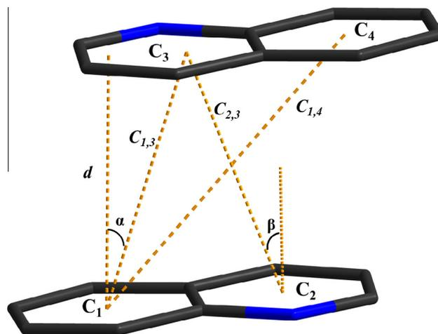
Fig. 3. Scheme for the parameters of  $\pi \cdots \pi$  interactions.  $d$ , the distance between the two  $\pi$  planes;  $C_{ij}$ , centroid-centroid distance of  $C_i$  and  $C_j$ ;  $\alpha$ ,  $\beta$ , the angle between the ring normal of quinoline plane and the centroid-centroid vector  $C_{1,3}$ ,  $C_{2,3}$ .
