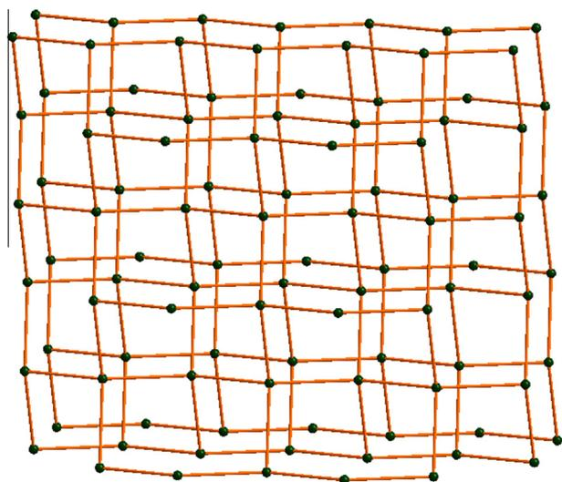
Fig. 2. The schematic representations of the uninodal 4-connected net of **1** and **2** with **dia** topology.
