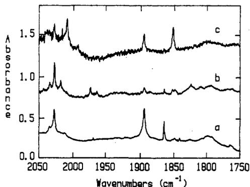
**Figure 2.** Infrared spectra in the 2150–1750-cm<sup>-1</sup> region after codeposition of uranium atoms for 3 h with 400:1 mixtures of argon and (a) <sup>12</sup>C<sup>16</sup>O, (b) <sup>12</sup>C<sup>16</sup>O, and (c) <sup>13</sup>C<sup>16</sup>O, and (c) <sup>12</sup>C<sup>16</sup>O and <sup>12</sup>C<sup>18</sup>O.
