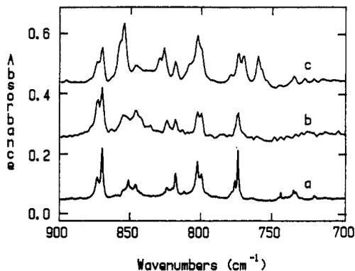
**Figure 4.** Infrared spectra in the 900–700-cm<sup>-1</sup> region for codeposition of uranium atoms for 3 h with mixtures of (a) 400/1 Ar/<sup>12</sup>C<sup>16</sup>O<sub>2</sub>, (b) 200/1 Ar/<sup>13</sup>C<sup>16</sup>O<sub>2</sub>, and (c) 300/1 Ar/<sup>12</sup>C<sup>16</sup>O<sub>2</sub>, Ar/<sup>12</sup>C<sup>16</sup>O<sup>18</sup>O, and Ar/<sup>12</sup>C<sup>18</sup>O<sub>2</sub>.
