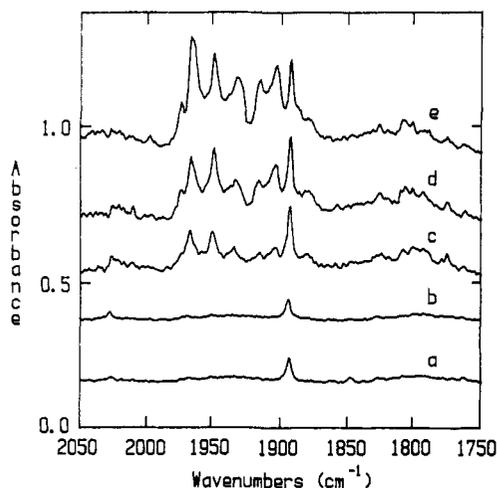
**Figure 3.** Infrared spectra in the 2150–1750-cm<sup>-1</sup> region for uranium atoms codeposited with a 600/1 Ar/CO sample at 12 K: (a) spectrum of sample codeposited for 4 h, (b) spectrum after 30 min of ultraviolet photolysis, (c) spectrum after a 12-21-12 K thermal cycle, (d) spectrum after a 12-25-12 K thermal cycle, and (e) spectrum after a 12-30-12 K thermal cycle.
