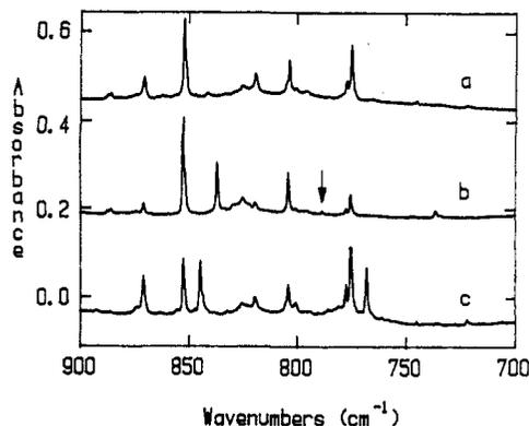
**Figure 1.** Infrared spectra in the 900–700-cm<sup>-1</sup> region for samples prepared by codeposition of uranium atoms for 3 h with 400:1 mixtures of argon and (a) <sup>12</sup>C<sup>16</sup>O, (b) <sup>12</sup>C<sup>16</sup>O and <sup>13</sup>C<sup>16</sup>O (arrow denotes <sup>13</sup>C<sup>16</sup>O absorption), and (c) <sup>12</sup>C<sup>16</sup>O and <sup>12</sup>C<sup>18</sup>O.
