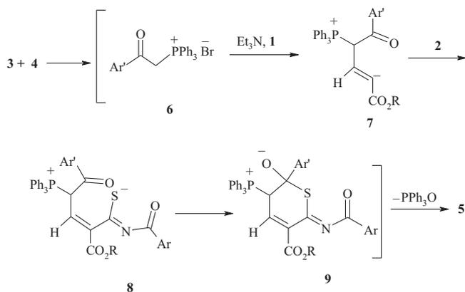
**Scheme 2.** Proposed mechanism for the synthesis of compound 5.
