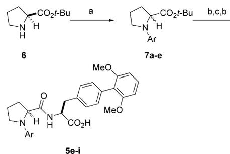
**Scheme 2.** (a) Aryl-halide, Pd<sub>2</sub>dba<sub>3</sub>, NaOtBu, BINAP, toluene, 80 °C; (b) TFA, CH<sub>2</sub>Cl<sub>2</sub>; (c) 2,6-dimethoxybiphenyl alanine *tert*-butyl ester, HATU, HOAt, *i*-Pr<sub>2</sub>NEt, CH<sub>2</sub>Cl<sub>2</sub>.
