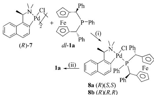
Reagents and conditions: (i) acetone, r.t., 2h, chromatographic separation of the diastereomeric complexes **8**; (ii) dppe,  $\text{CH}_2\text{Cl}_2$ , r.t., 3h
