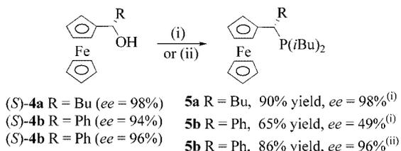
Reagents and conditions: (i) slow addition of *i*Bu<sub>2</sub>PH (1 equiv.) to a solution of **4** in AcOH, at r.t. (ii) rapid addition of *i*Bu<sub>2</sub>PH (1 equiv.) to an ice-cooled suspension of **4** in AcOH.
