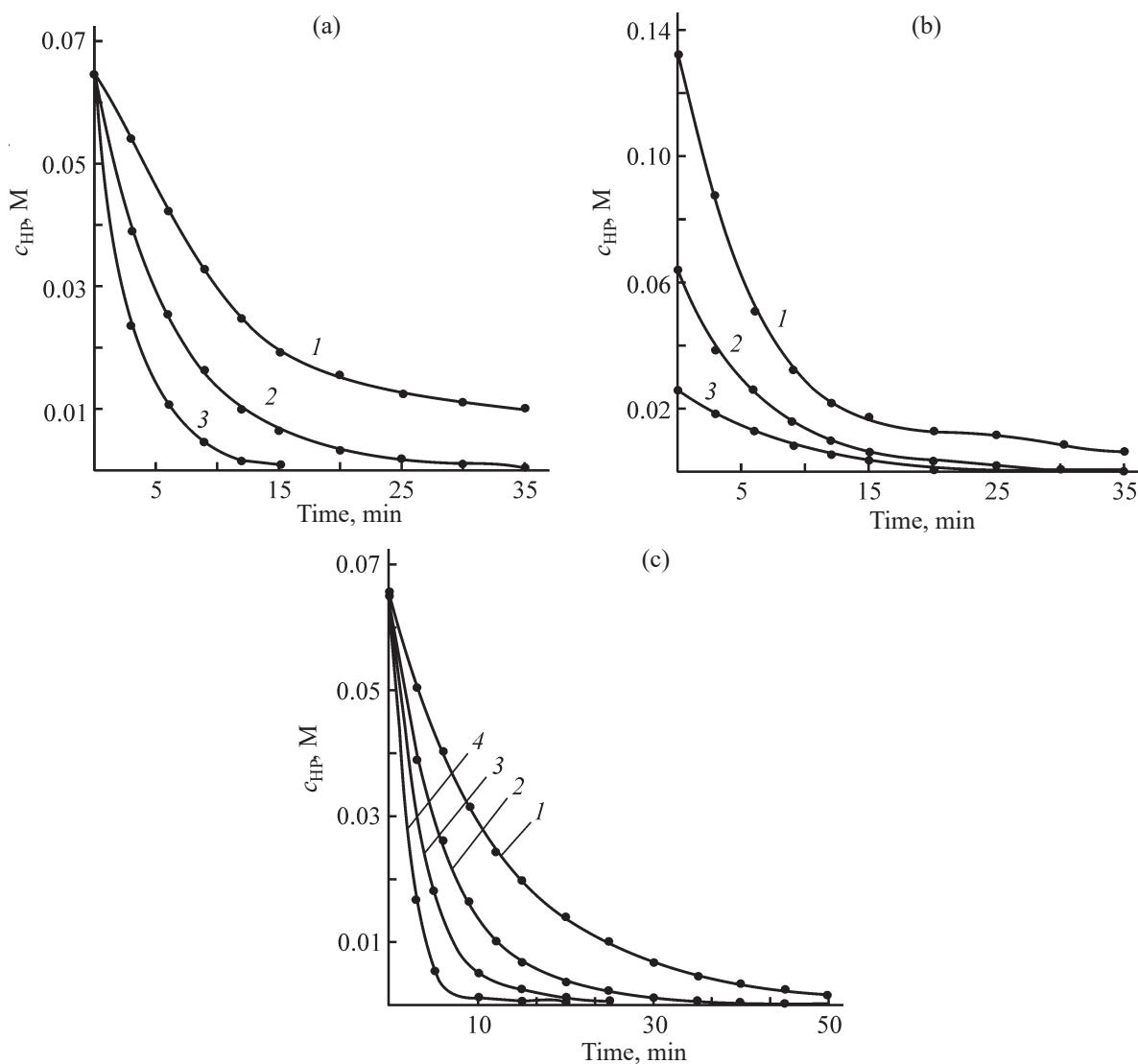
**Fig. 2.** Kinetic relationships of the acid decomposition of *p*-*tert*-butylcumene hydroperoxide under various conditions. (a) Temperature, °C: (1) 30, (2) 40, and (3) 50; catalyst concentration 0.6 wt %. (b) Initial hydroperoxide concentration, M: (1) 0.132, (2) 0.065, and (3) 0.026; temperature 40°C; catalyst concentration 0.6 wt %. (c) Catalyst concentration, wt %: (1) 0.3, (2) 0.6, (3) 0.9, and (4) 1.5; temperature 40°C.
