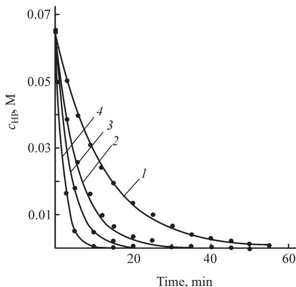
**Fig. 3.** Kinetic curves of acid decomposition of *p*-*tert*-butylcumene hydroperoxide at various catalyst concentrations. Curves: calculation using Eq. (7); points: experimental data. Catalyst (concentrated H<sub>2</sub>SO<sub>4</sub>) concentration, wt %: (1) 0.3, (2) 0.6, (3) 0.9, and (4) 1.5.
