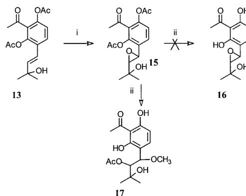
**Figure 5** Oxidation of compound **13** followed by deacetylation, to produce the diphenol **17** instead of the expected epoxyphenol **16**. Reagents: i, mCPBA,  $\text{CH}_2\text{Cl}_2$ , RT; ii, Zn,  $\text{MeOH}-\text{CH}_2\text{Cl}_2$ .
