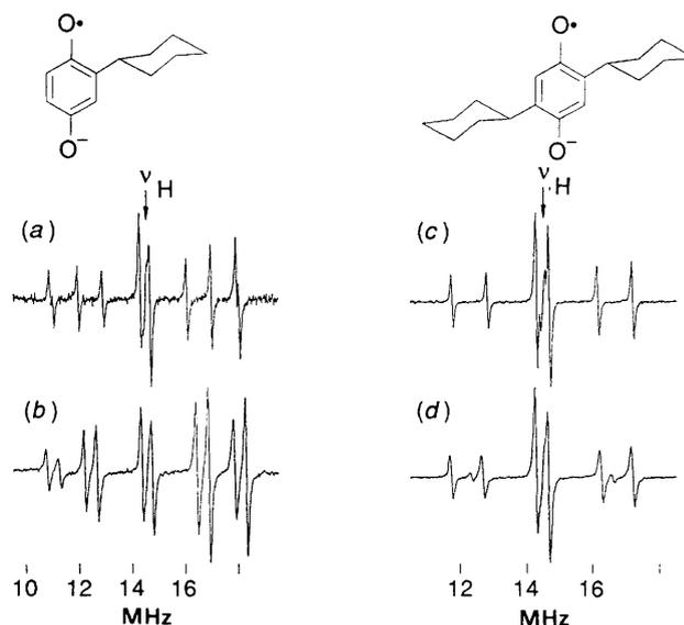
**Fig. 3.** ENDOR spectra of (a)  $5^{\cdot-}$  in propan-2-ol at 300 K, (b)  $5^{\cdot-}$  in reversed-micellar solution [cf. fig. 2(b)] at 300 K, (c)  $6^{\cdot-}$  in propan-2-ol at 300 K and (d)  $6^{\cdot-}$  in reversed-micellar solution at 330 K,  $W_0 = 15$ .
