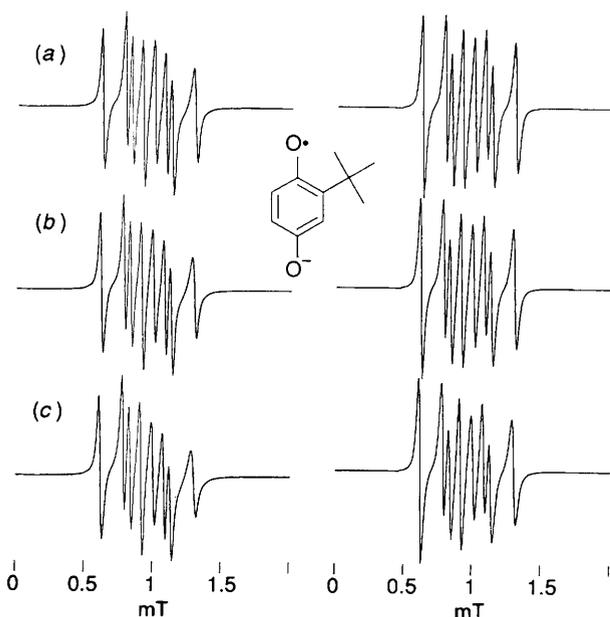
Fig. 5. EPR spectra of  $4^{\bullet-}$  in reversed-micellar solution,  $0.3 \text{ mol dm}^{-3}$  CTAB,  $\text{CHCl}_3$ -*n*-heptane (1 : 1),  $1 \text{ mol dm}^{-3}$  LiOH,  $W_0 = 10$ , at different temperatures: (a) 300, (b) 290, (c) 280 K. In each case, the left trace is the experimental spectrum; the right trace is the computer-simulated spectrum.
