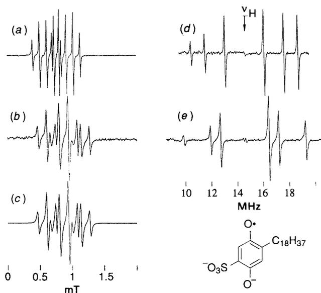
**Fig. 4.** EPR and ENDOR spectra of  $7^{\bullet-}$ . EPR: (a) in propan-2-ol at 290 K; (b) in reversed-micellar solution, 0.2 mol dm<sup>-3</sup> CTAB, 2-methylhexan-2-ol-cyclohexane (1 : 5), 1 mol dm<sup>-3</sup> KOH, 1 mol dm<sup>-3</sup> KBr,  $W_0 = 20$ , 290 K; (c) computer simulation. ENDOR (d) in propan-2-ol at 290 K and (e) in reversed-micellar solution at 290 K.
