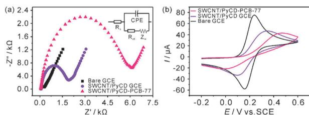
**Fig. 1** Nyquist diagram of electrochemical impedance spectra (a) and cyclic voltammograms (b) of a bare GCE, SWCNT/PyCD GCE and SWCNT/PyCD after preconcentration of 10  $\mu\text{M}$  PCB-77 in the solution of 5 mM  $\text{Fe}(\text{CN})_6^{3-/4-}$  and 0.1 M KCl. The inset in panel (a) is an equivalent circuit of the SWCNT/PyCD electrochemical impedance measurement system (see ESI† for details). In panel (b), scan rate is 50  $\text{mV s}^{-1}$ .
