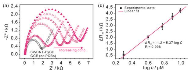
**Fig. 2** (a) Nyquist diagram of electrochemical impedance spectra of a SWCNT/PyCD GCE before and after preconcentration of a range of concentrations (2, 4, 6, 8 and 10  $\mu\text{M}$ ) of PCB-77. (b) Plot of  $\Delta R_{\text{ct}}$  as a function of logarithmic value of PCB-77 concentrations shown in panel (a).
