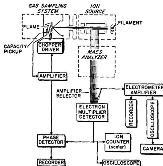
FIG. 6. Block diagram of the mass spectrometer.
