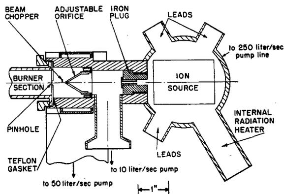
FIG. 2. Cross section of mass spectrometer gas inlet system.
