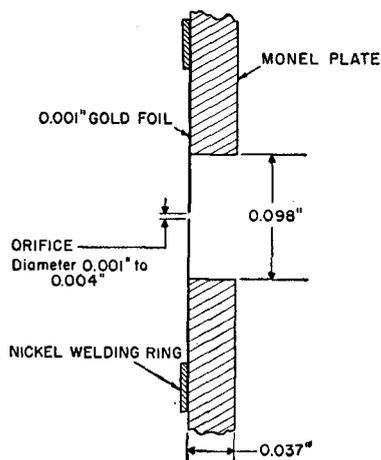
FIG. 4. Sampling orifice construction.
