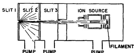
FIG. 1. Schematic diagram of the molecular beam gas sampling system.
