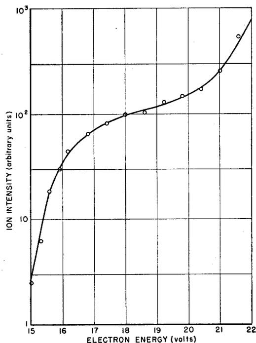
FIG. 9. Appearance potential curve for the OH radical in the hydrogen-oxygen flame. Voltages are uncorrected for contact potentials, space charge, etc.
