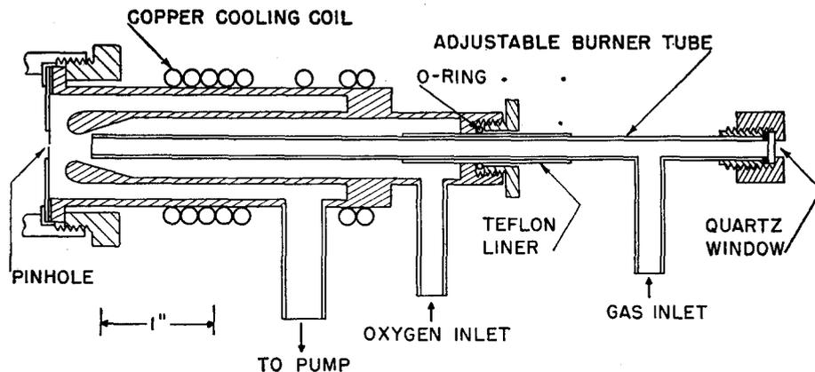
FIG. 3. Burner assembly.
