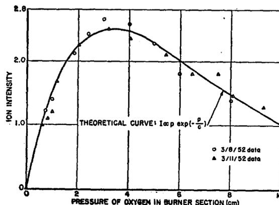
FIG. 5. Beam intensity as a function of pressure in the burner section.
