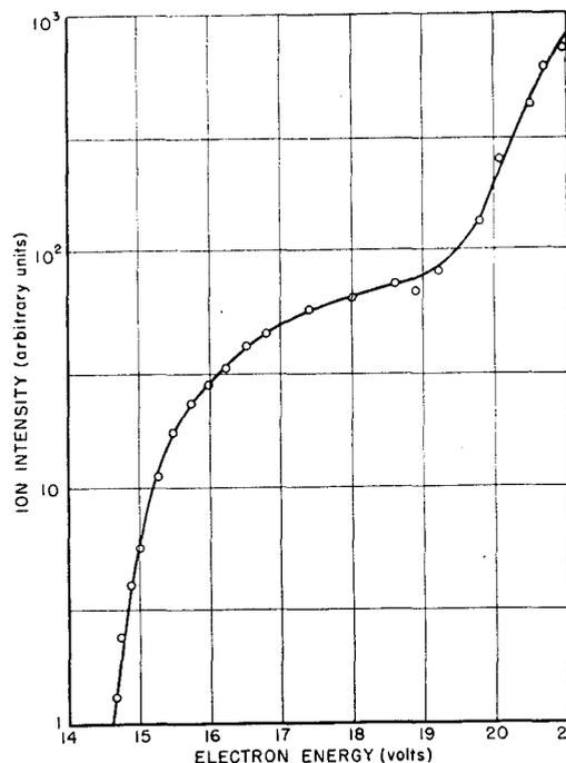
Fig. 8. Appearance potential curve for hydrogen atoms in the hydrogen-oxygen flame. Voltages are uncorrected for contact potentials, space charge, etc.
