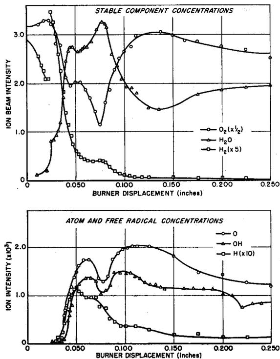
FIG. 10. Ion intensity measurements of stable components and intermediates in the low pressure hydrogen-oxygen flame. The abscissa is the relative displacement of the central burner tube from the pinhole.
