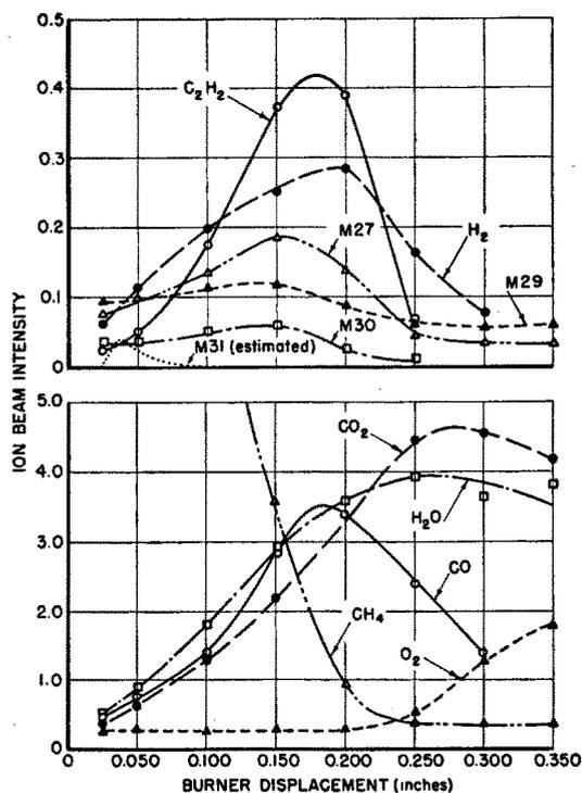
FIG. 11. Ion intensity measurements of the major components in a low pressure methane-oxygen flame. The data were obtained by photographing oscilloscope presentations of the mass spectra and are uncorrected for background. The abscissa is the relative displacement of the burner tube from the pinhole.
