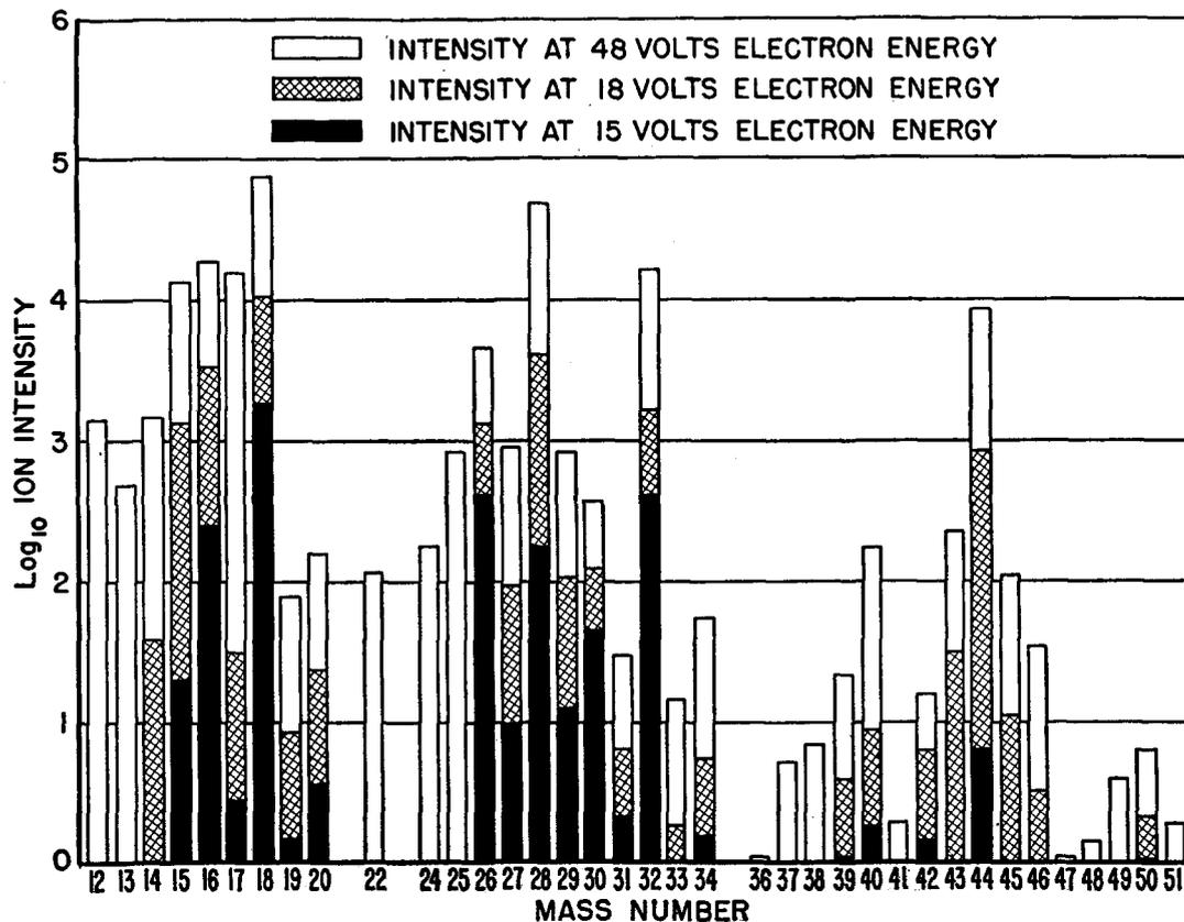
FIG. 12. Mass spectra of the methane-oxygen flame obtained at different values of electron energy. A range of  $10^6$  in intensities is covered by the logarithmic scale. The actual electron energies are lower than the indicated voltages by about 1.5 volts because of contact potentials, space charge, etc.
