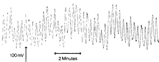
**Figure 2.** A train of oscillations in electrode potential in the CSTR reactor with residence time 48 min. Concentrations which would have existed in the reactor if there had been no chemical change were  $[\text{BrO}_3^-] = 0.033 \text{ M}$ ,  $[\text{Na}_2\text{S}] = 0.001 \text{ M}$ ,  $[\text{HClO}_4] = 0.05 \text{ M}$ .
