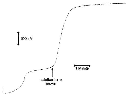
**Figure 1.** Trace of the potential of a platinum electrode in a batch reactor. Composition at time zero was  $[\text{BrO}_3^-] = 0.03 \text{ M}$ ,  $[\text{Na}_2\text{S}] = 8 \times 10^{-4} \text{ M}$ ,  $[\text{HClO}_4] = 0.05 \text{ M}$ . Note the two autocatalytic rises.
