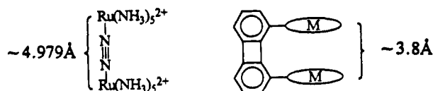
Figure 9. A comparison of the metal-metal distance in the bridged dinitrogen complex [(\text{NH}_3)_5\text{RuNNRu}(\text{NH}_3)_5]^{4+} to the distance between the two metals found in the biphenylene bridged cofacial diporphyrins. 17a,23,36
