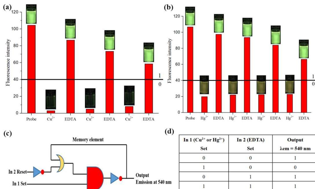
**Fig. 12** (a) bar diagram represents input (In 1 = Cu<sup>2+</sup> and In 2= EDTA ) and output emissions (at 40 au); (b) bar diagram represents input (In 1 = Hg<sup>2+</sup> and In 2= EDTA ) and output emissions (at 40 au); (c) IMPLICATION logic gate with two inputs (In 1 and In 2) and one output; (d) corresponding truth table.
