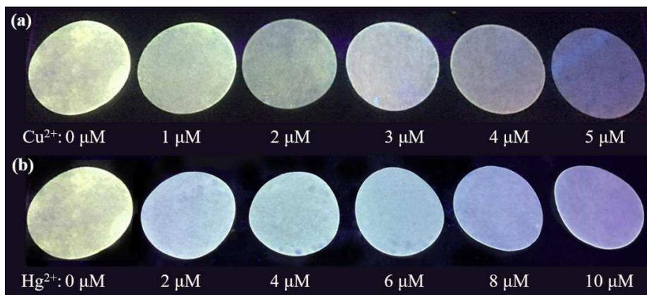
**Fig. 11** The photographs of probe BHMB on test strips with different concentrations of (a)  $\text{Cu}^{2+}$  and (b)  $\text{Hg}^{2+}$  at room temperature under 365 nm UV light, respectively.
