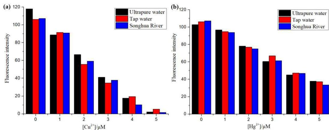
**Fig. 10** Fluorescent detection of BHMB (10  $\mu\text{M}$ ) in “ultrapure water”, “tap water”, and “Songhua River” upon addition of different concentration of (a)  $\text{Cu}^{2+}$  and (b)  $\text{Hg}^{2+}$ , respectively. The data was obtained at 540 nm.
