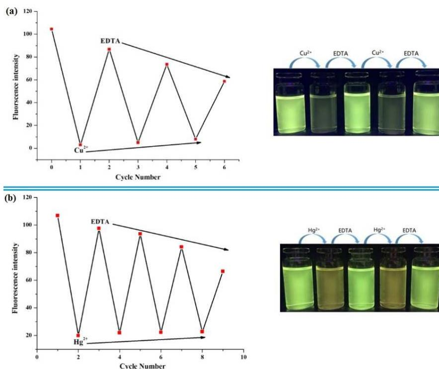
**Fig. 9** (a) Reversible changes in color and fluorescence intensity of BHMB (10  $\mu\text{M}$ ) at 540 nm in DMF/ $\text{H}_2\text{O}$  (3/7, v/v, 0.01M HEPES, pH = 7.0) upon alternate addition of  $\text{Cu}^{2+}$  and EDTA; (b) Reversible changes in color and fluorescence intensity of BHMB (10  $\mu\text{M}$ ) at 540 nm in DMF/ $\text{H}_2\text{O}$  (3/7, v/v, 0.01M HEPES, pH = 7.0) upon alternate addition of  $\text{Hg}^{2+}$  and EDTA.
