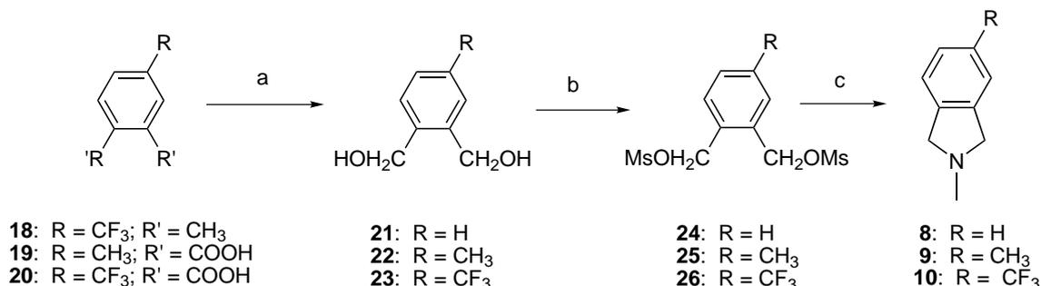
Scheme 3. Synthetic pathway to the isoindolines **8–10**. (a) LiAlH<sub>4</sub>, THF; (b) MsCl, NEt<sub>3</sub>; (c) MeNH<sub>2</sub>.
