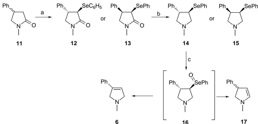
Scheme 2. Synthetic pathway to 1-methyl-4-phenyl-3-pyrroline (**6**). (a) i. LDA, THF, ii. PhSeCl; (b) BH<sub>3</sub>·THF, THF; (c) H<sub>2</sub>O<sub>2</sub> 30%.
