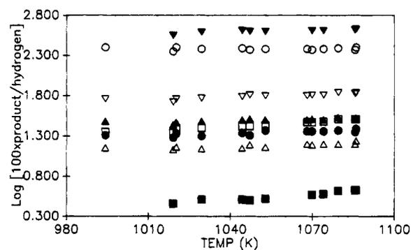
**Figure 2.** Product distributions from the hydrogen-atom-induced decomposition of trichloroethylene as a function of temperature. Reaction mixture contains 100 ppm hexamethylethane, 20% hydrogen, 2% trichloroethylene, and 1% mesitylene in argon. (▼) Sum of products, (○) 1,1-dichloroethylene, (▽) 2,4-dimethylbenzyl [calculated], (▲) *m*-xylene, (□) chloroacetylene, (●) *trans*-1,2-dichloroethylene, (△) *cis*-1,2-dichloroethylene, and (■) dichloroacetylene. Pressures are from 2 to 6 atm.
