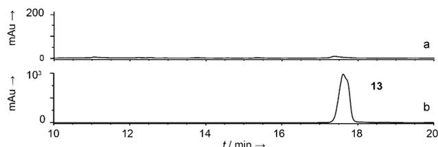
**Figure 2.** Mutasynthesis of the vinyl-substituted chartreusin analogue **13**. HPLC profiles ( $\lambda = 400$  nm) of extracts from cultures of  $\Delta$ PKS mutant supplemented with the following substrates: a) DMSO (negative control), b) synthetic vinylchartarin (**12**) in DMSO.
