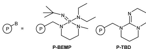
**Figure 1.** Structure of polymer-bound BEMP.
