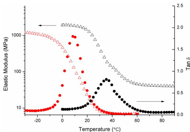
**Figure 5.** Plots of  $\tan \delta$  and elastic modulus vs temperature for two stage networks formed through thiol–acrylate–methacrylate monomer cross-linking (PETMA–TMPTA–TMPTMA, molar ratio = 3:2:2) system. Stage 1 (predominately the thiol–acrylate cross-linking reaction) data are in red and stage 2 (the subsequent thiol–methacrylate cross-linking reaction) data are in black.
