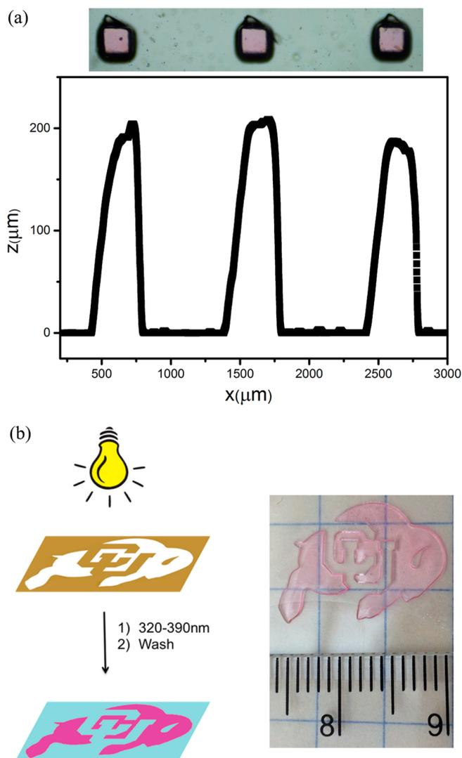
**Figure 3.** Photopatterning with 320–390 nm (20 mW/cm<sup>2</sup>) light of a tetra-thiol (PETMA) and trimethacrylate (TMPTMA) thiol–Michael addition monomer system (1 mol % rhodamine B-modified acrylate was used as dye to provide contrast). Key: (a) Cubic size: width ~ 400 μm, height ~ 200 μm. (b) The width of the CU buff logo is ~ 16 μm.
