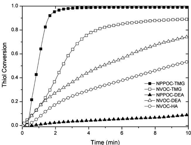
**Figure 1.** Thiol conversion versus time monitored by FT-IR for the model reaction between thiol glycolate and ethyl acrylate with 5 mol % photolabile catalyst irradiated using a Hg light source equipped with 320–390 nm (20 mW/cm<sup>2</sup>) (filled square, NPPOC-TMG; open square, NVOC-TMG; filled triangle, NPPOC-DEA; open triangle, NVOC-DEA; open circle, NVOC-HA).
