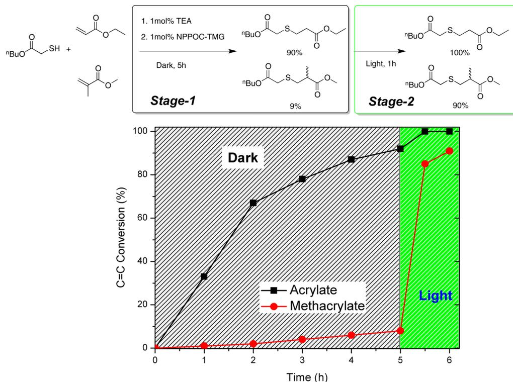
**Figure 4.** C=C conversion of thiol–acrylate (stoichiometric mixture of butyl thiol glycolate and methyl acrylate with 1 mol % TEA) and thiol–methacrylate (stoichiometric mixture of butyl thiol glycolate and ethyl methacrylate with 1 mol % NPPOC-TMG) monitored by <sup>1</sup>H NMR.
