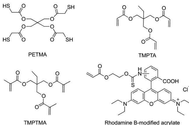
**Figure 2.** Monomers used for polymer networks formation.
