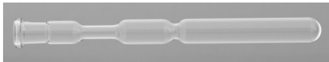
Figure 7. Rendered 3D sketch of the ampoule used for the synthesis of thorium(IV) halides.
