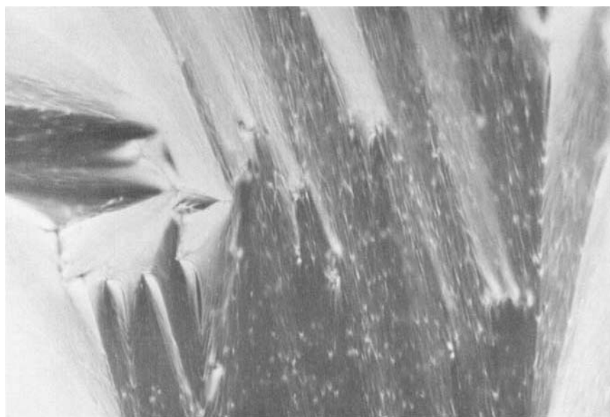
PLATE 5 Focal-conic fan texture of the smectic A phase of the contact region between N -(4'- n -butyloxybenzylidene)-4- n -octylaniline (left) and n -hexyl 4'-pentyloxybiphenyl-4-carboxylate (right), showing parabolic focal-conic defects ( \times 100 ).
