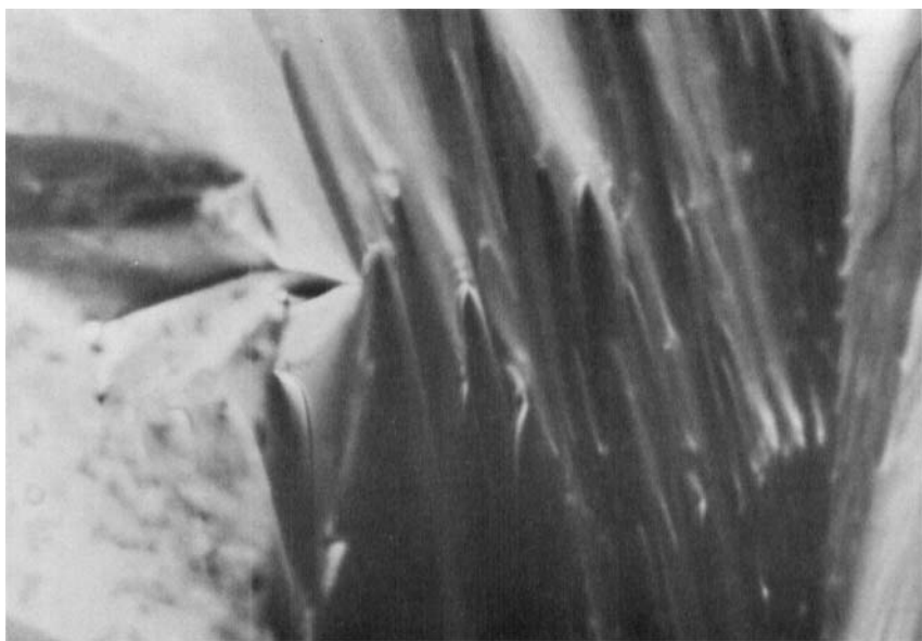
PLATE 6 The N—S A transition 'barrier' as it crosses the contact region so destroying the parabolic focal-conic defects. The contact preparation is between N -(4'- n -butyloxybenzylidene)-4- n -octylaniline (left) and n -hexyl 4'- n -pentyloxybiphenyl-4-carboxylate (right) (×100).
