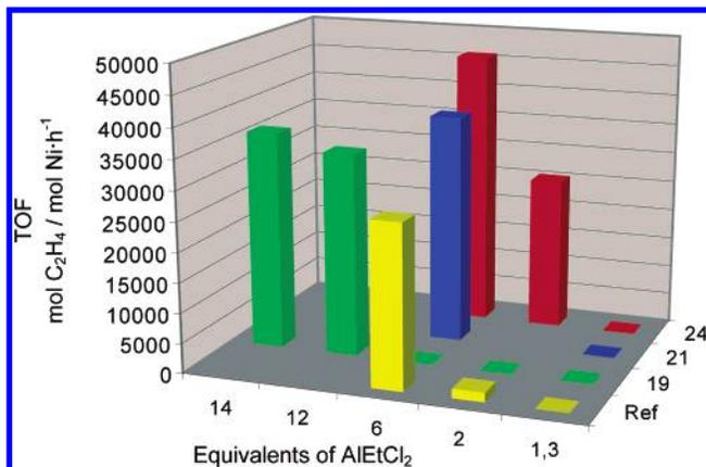
**Figure 5.** Catalytic activities of the complexes **19**, **21**, and **24** in the oligomerization of ethylene using AlEtCl<sub>2</sub> as activator ([NiCl<sub>2</sub>(PCy<sub>3</sub>)<sub>2</sub>] reference). Conditions: *T* = 30 °C, 10 bar of C<sub>2</sub>H<sub>4</sub>, 35 min, 4 × 10<sup>-2</sup> mmol of Ni, 15 mL of toluene.
