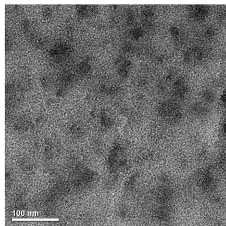
**Fig. 1** TEM image of  $Pd^{2+}$ -stained membrane: PES-G-OH, IEC = 1.39 meq/g.
