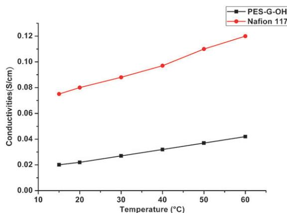
**Fig. 2** Temperature dependence of the hydroxide ion conductivity of the membranes.
