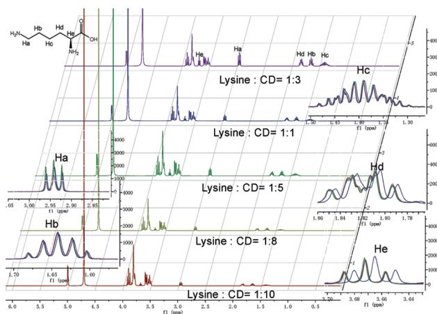
**Figure 3.**  $^1\text{H}$  NMR (400-MHz) spectra in  $\text{D}_2\text{O}$  at 298K of  $\beta$ -CD ( $10^{-3}\text{mol}\cdot\text{L}^{-1}$ ) upon addition of L-lysine. Chemical shifts ( $\delta$ ) are reported in ppm and referenced to the residual solvent peak as an internal standard ( $\delta=4.7000\text{ppm}$  for  $^1\text{H}$  NMR in  $\text{D}_2\text{O}$ ). (Figure is provided in color online.)
