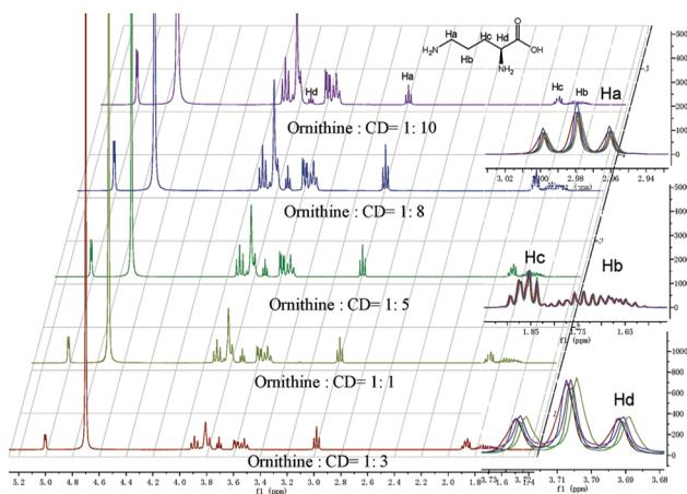
**Figure 4.**  $^1\text{H}$  NMR (400 MHz) spectra in  $\text{D}_2\text{O}$  at 298K of  $\beta$ -CD ( $10^{-3} \text{ mol} \cdot \text{L}^{-1}$ ) upon addition of L-ornithine. Chemical shifts ( $\delta$ ) are reported in ppm and referenced to the residual solvent peak as an internal standard ( $\delta = 4.7000 \text{ ppm}$  for  $^1\text{H}$  NMR in  $\text{D}_2\text{O}$ ). (Figure is provided in color online.)
