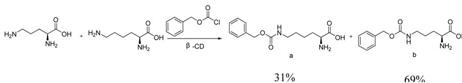
**Scheme 2.** Chemoselectivity between L-lysine and L-ornithine in the presence of  $\beta$ -CD. Conversion determined from  $^1\text{H}$  NMR spectrum of crude reaction mixture.
