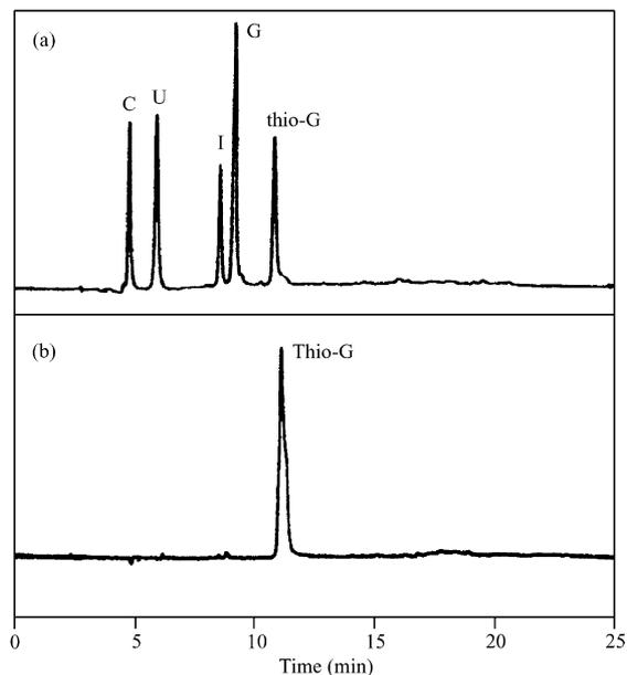
**Figure 3.** Nucleoside composition analysis<sup>26</sup> of  $5'$ -GCG<sup>SH</sup> AU-3'. The nucleosides generated from digestion with snake venom phosphodiesterase and alkaline phosphatase were separated by HPLC with monitoring at (a) 260 nm; and at (b) 345 nm. The identity of the peaks was confirmed by retention time comparison with the authentic samples. Inosine was resulted from the deamination of adenosine by adenosine deaminase, which is a contaminant in the enzyme preparations.
