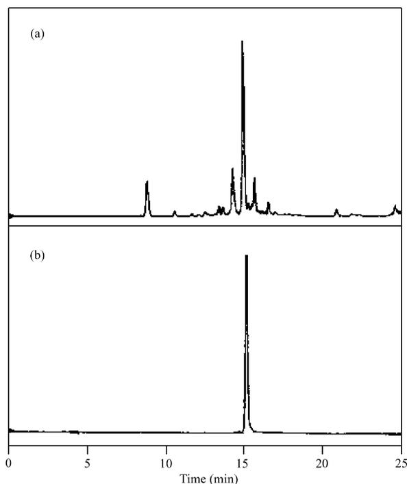
**Figure 1.** The reverse phase HPLC chromatograms of the oligoribonucleotide  $5'$ -GCG<sup>SH</sup> AU-3'. (a) After Nen-sorb column purification; (b) after further purification with HPLC. C18 columns were used with 0.1 M triethylammonia acetate, pH 6.5, and acetonitrile gradients of 2–20% over 25 min at a flow rate of 1 mL/min, recorded at 260 nm.
