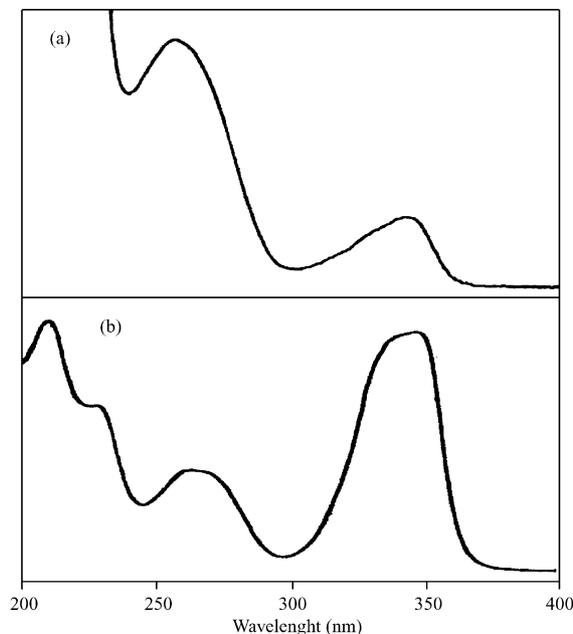
**Figure 2.** UV spectrum of the oligoribonucleotide  $5'$ -GCG<sup>SH</sup> AU-3' showing peaks at (a) 260 and 346 nm; and (b) that of 6-thioguanosine showing a major peak at 343 nm.
