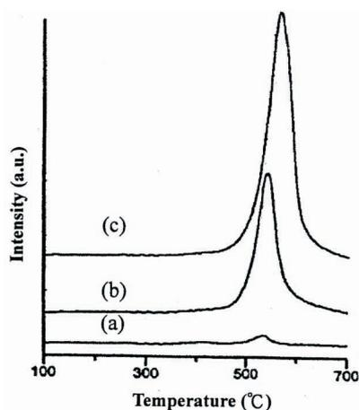
Fig. 4. TPR of hydrogen profiles from various calcined samples. (a) Si-MCM-41; (b) 4 V-MCM-41; (c) 9V/MCM-41.
