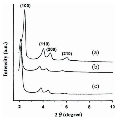
Fig. 1. The low angle XRD patterns of various calcined samples. (a) Si-MCM-41; (b) 4 V-MCM-41; (c) 9 V/MCM-41.
