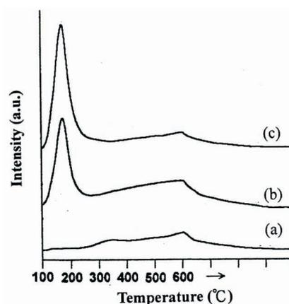
Fig. 3. TPD of ammonia profiles from various calcined samples. (a) Si-MCM-41; (b) 4 V-MCM-41; (c) 9 V/MCM-41.
