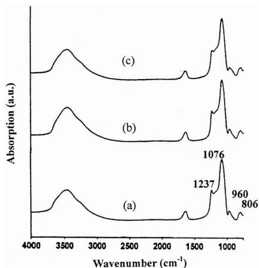
Fig. 2. FT-IR spectra of various calcined samples. (a) Si-MCM-41; (b) 4 V-MCM-41; (c) 9 V/MCM-41.
