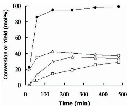
Fig. 5. The influence of reaction time on the conversion and product yields in the oxidation of 9,10-dihydroanthracene over 4 V-MCM-41. (●) conversion; yield: (○) anthrone; (Δ) anthraquinone; (□) anthracene.
