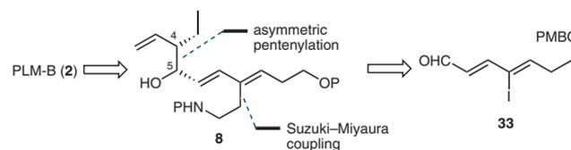
Scheme 7 Synthetic plan for the preparation of key intermediate **8**
