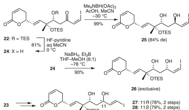
Scheme 5 Preparation of pivotal intermediates
