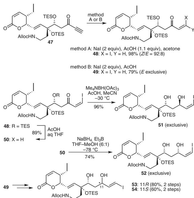
Scheme 11 Preparation of advanced intermediate **51** and its isomers
