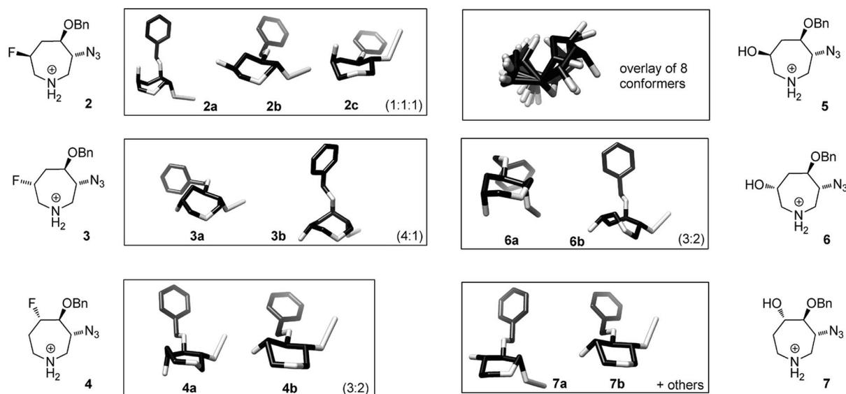
Figure 2. Conformations of azepanes 2–7. Only the major conformer of azepane 3 simultaneously satisfies the C3/C4 pseudo-diequatorial preference, the azido *gauche* effect and the fluorine *gauche* effect.
