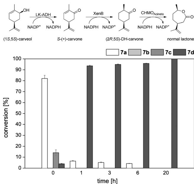
**Figure 3.** *In vivo* cascade for the conversion of (1*S*,5*S*)-carveol (**7a**) into corresponding lactone **7d**.
