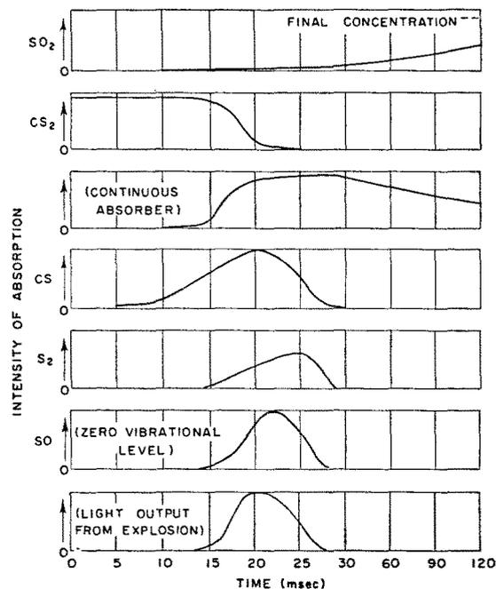
FIG. 2. Occurrence of free radicals and molecules during the  $\text{CS}_2\text{-O}_2$  explosion. These curves represent estimated absorption intensities as a function of time, as determined from several hundred experiments.
