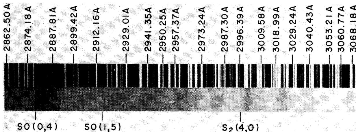
FIG. 4(c). Absorption spectrogram of CS<sub>2</sub>-O<sub>2</sub> explosion, 2862-3068 Å.
