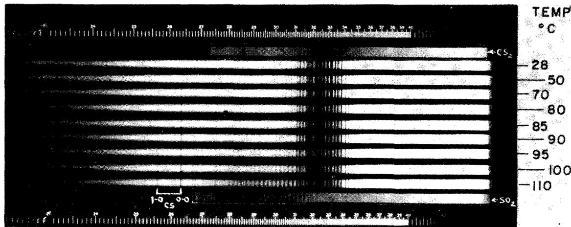
FIG. 3. Growth of CS and SO<sub>2</sub> in a nonexploding mixture of 25 mm of Hg of CS<sub>2</sub> and 75 mm of Hg of O<sub>2</sub> at temperatures of 28° to 110°C. The CS quickly attains a constant (steady-state) concentration which is an increasing function of temperature, while the SO<sub>2</sub> concentration increases with time.
