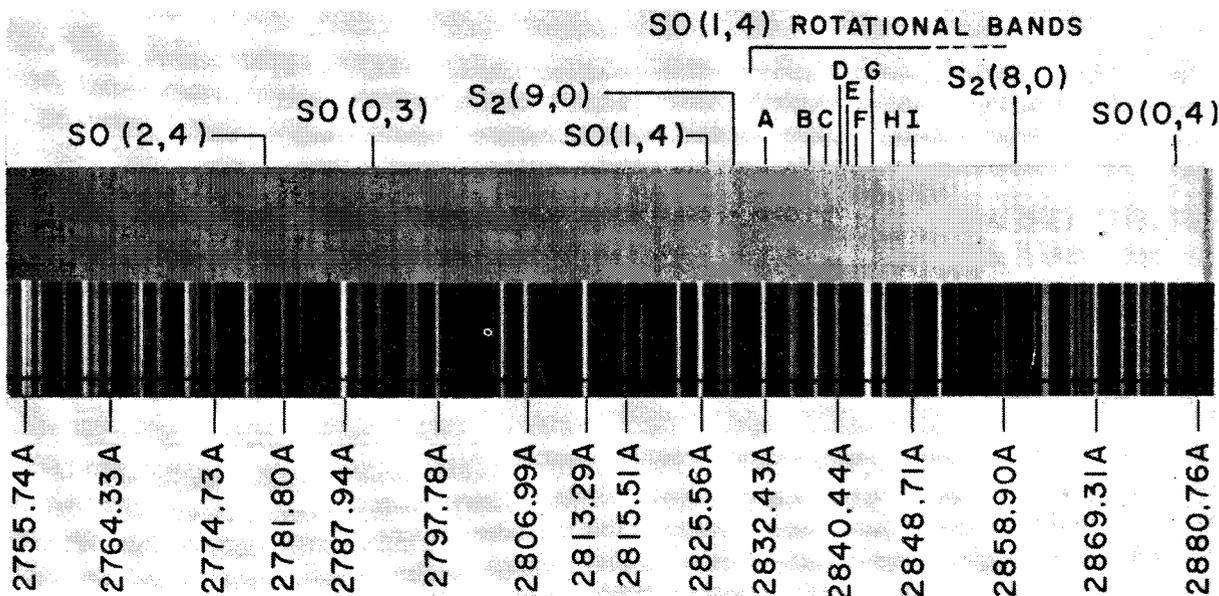
Fig. 4. (b) Absorption spectrogram of  $\text{CS}_2\text{-O}_2$  explosion, 2756–2880 Å.
