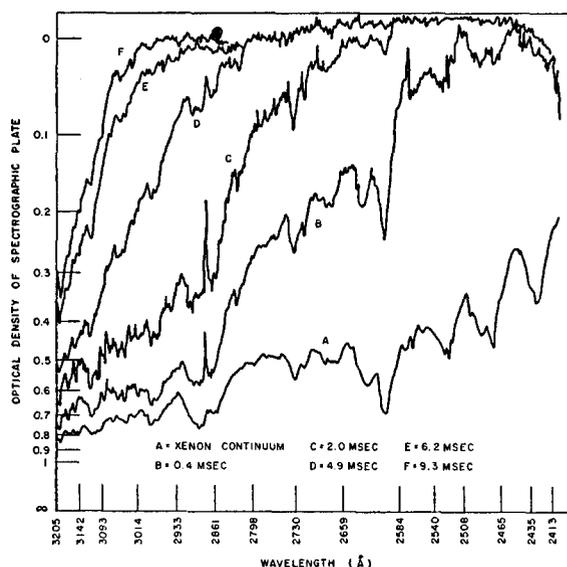
FIG. 6. Microphotometer traces of absorption spectra showing growth of continuous absorber during 1:3 CS<sub>2</sub>:O<sub>2</sub> explosions (total pressure = 35 mm Hg). The time, in milliseconds, after the beginning of light emission at which each spectrum was taken is given by B through F.
