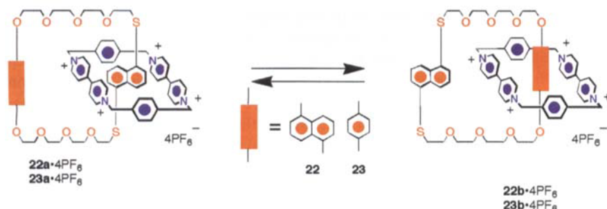
Figure 14. Translational isomers associated with the [2]catenanes 22 ·4PF 6 and 23 ·4PF 6 .
