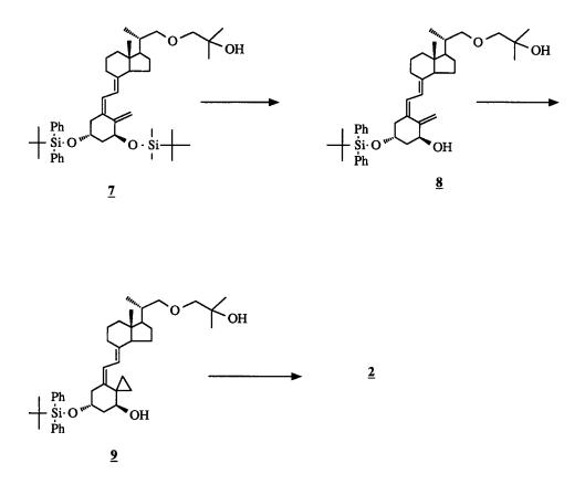
We made use of the different chemical stabilities observed for silyl ethers as protecting groups. Whereas a tert.butyl-diphenyl silyl ether remains stable under the conditions of mild acid treatment (1n-HCl, methanol, 25°C), a tert.-butyl-dimethyl silyl ether becomes smoothly cleaved.
