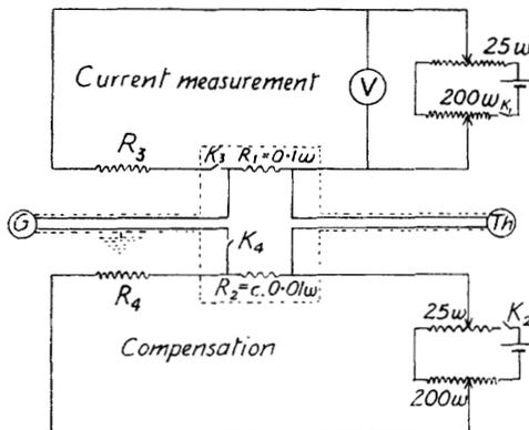
FIG. 3.—The thermopile circuit.
