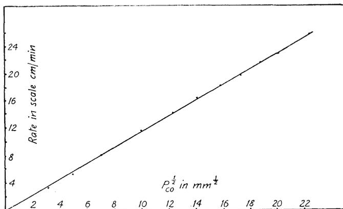
FIG. 6.—Variation of the rate with carbon monoxide pressure.
