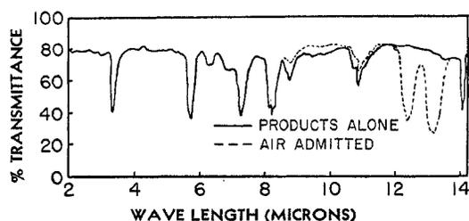
Figure 1. Decomposition products of *tert*-butyl nitrite ( $P_o = 35$  mm.) at  $181^\circ\text{C}$ ,  $t = 1020$  minutes
