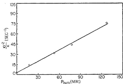
Figure 5. Effect of nitric oxide on thermal decomposition of *tert*-butyl nitrite at 201° C.
