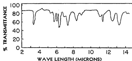
Figure 2. Decomposition products of *tert*-butyl nitrite ( $P_o = 36$  mm.) in presence of nitric oxide ( $P_o = 65$  mm.) at  $181^\circ\text{C}$ ,  $t = 1022$  minutes
