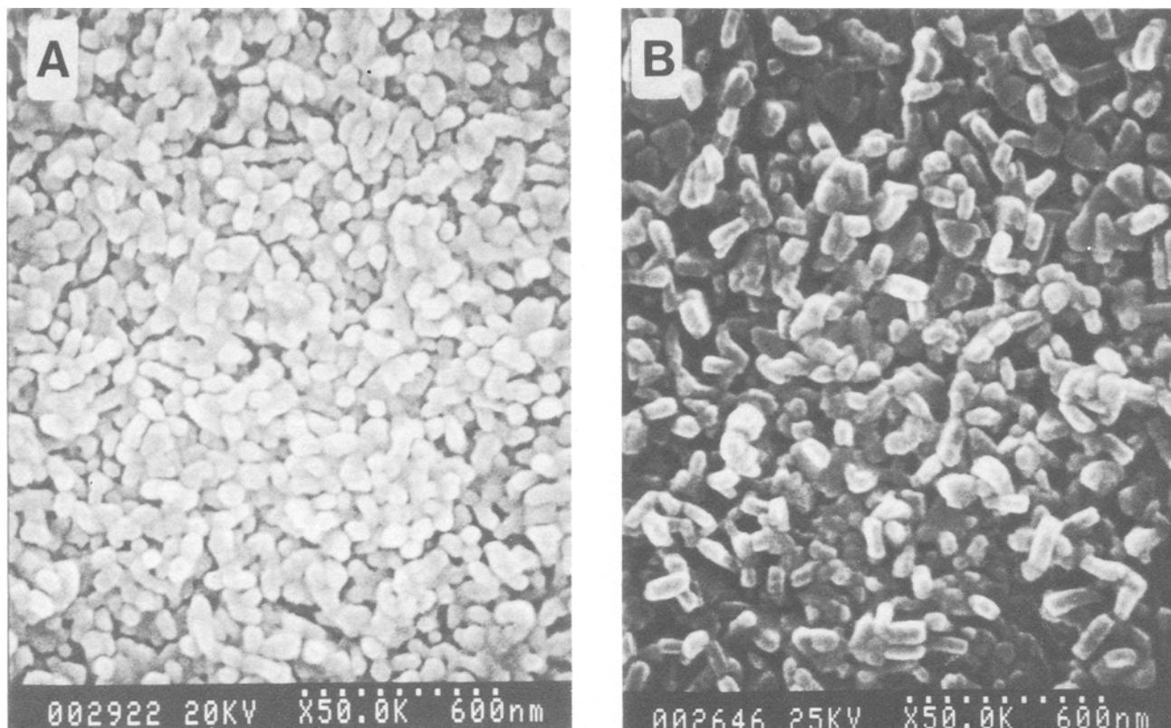
Fig. 10. Scanning electron micrograph of a 0.26  $\mu\text{m}$  thick CIAIPc film after transformation I (A) and a 0.30  $\mu\text{m}$  thick CIAIPc film, after transformation H (B).
