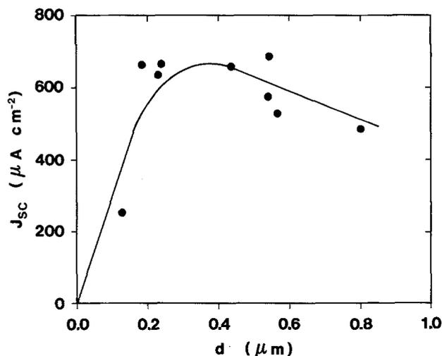
Fig. 4. Variation of  $J_{sc}$  (white light illumination at  $35 \text{ mW cm}^{-2}$ ) as a function of the thickness of CIAIPc after completion of transformation I.
