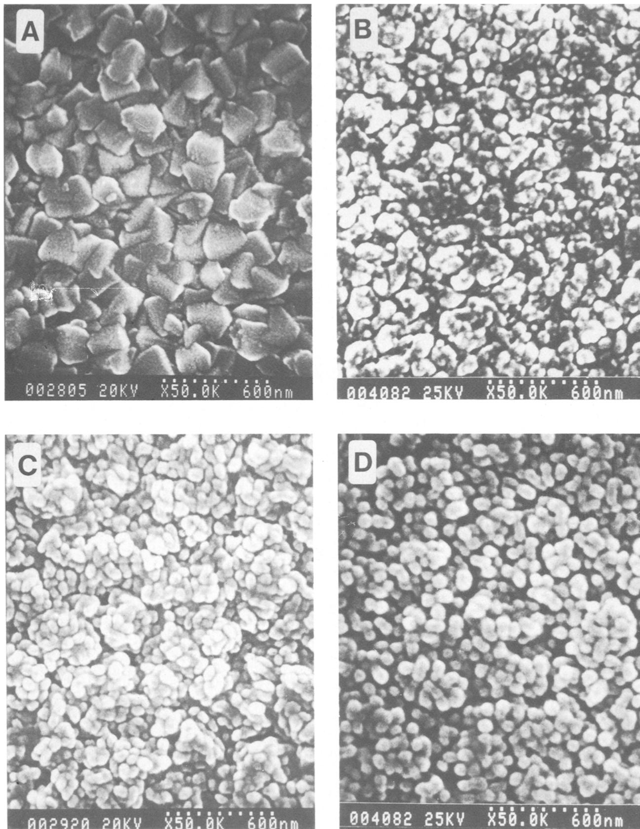
Fig. 9. Scanning electron micrograph of the  $\text{SnO}_2$  substrate (A), of a 0.10 (B), 0.24 (C), and 0.60  $\mu\text{m}$  thick CIAIPc film, (D)
