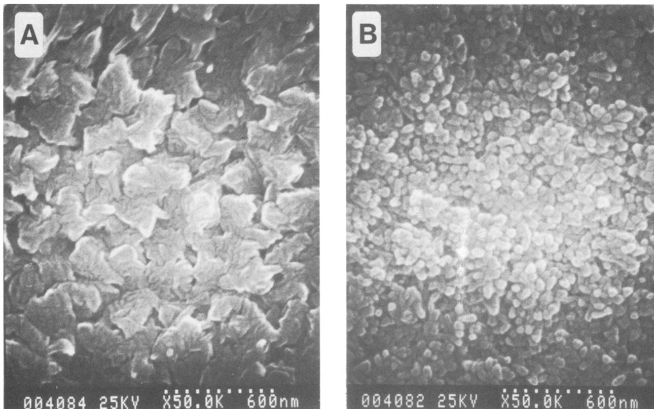
Fig. 12. Scanning electron micrograph of a 0.12  $\mu\text{m}$  thick FAIPc film (A) and a 0.32  $\mu\text{m}$  thick PcAlOAlPc film (B)
