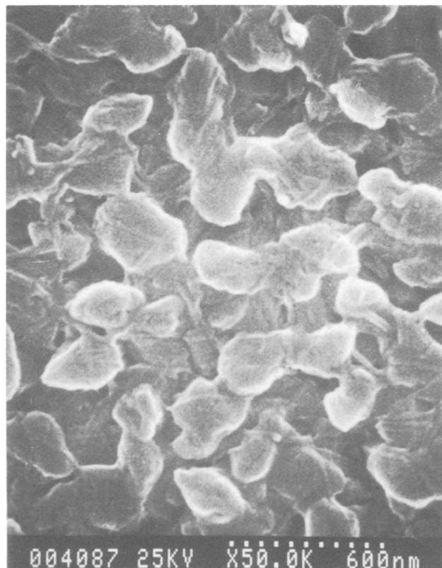
Fig. 11. Scanning electron micrograph of a 0.15  $\mu\text{m}$  thick CIAIPc film slowly grown on a hot substrate.
