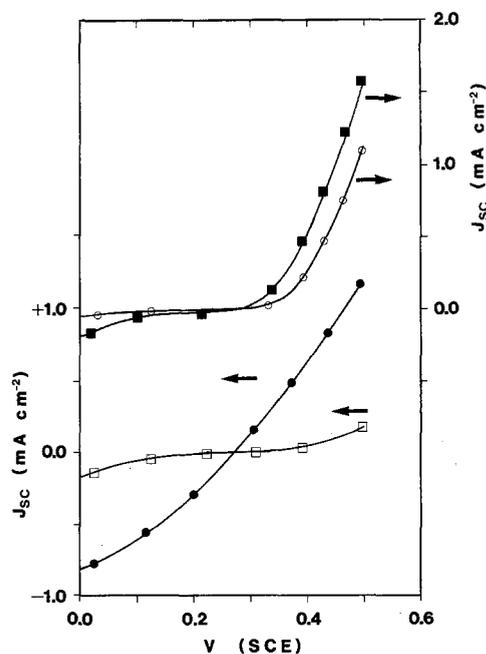
Fig. 8. Dark J-V characteristics of a CIAIPc film before (○) and after transformation I (■); of a FAIPc film (●); of bare  $\text{SnO}_2$  substrate (□). The redox is  $\text{I}_3^-/\text{I}^-$  at pH 3.2.
