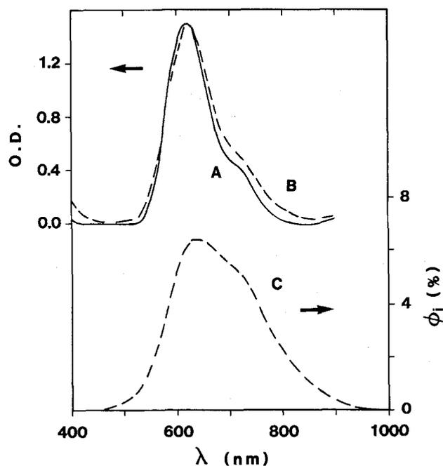
Fig. 6. Absorption spectra (curves A and B) and incident quantum efficiencies,  $\phi_i$  (curve C) of a  $0.32 \mu\text{m}$  thick  $\text{PcAlOAlPc}$  film; before (A) and after transformation I (B and C).
