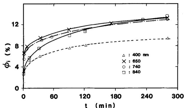
Fig. 3. Time evolution, during transformation I, of  $\phi_i$  at 400 nm ( $\Delta$ ), 650 nm (X), 740 nm ( $\circ$ ), and 840 nm ( $\square$ ), for a 0.6  $\mu\text{m}$  thick ClAlPc film.
