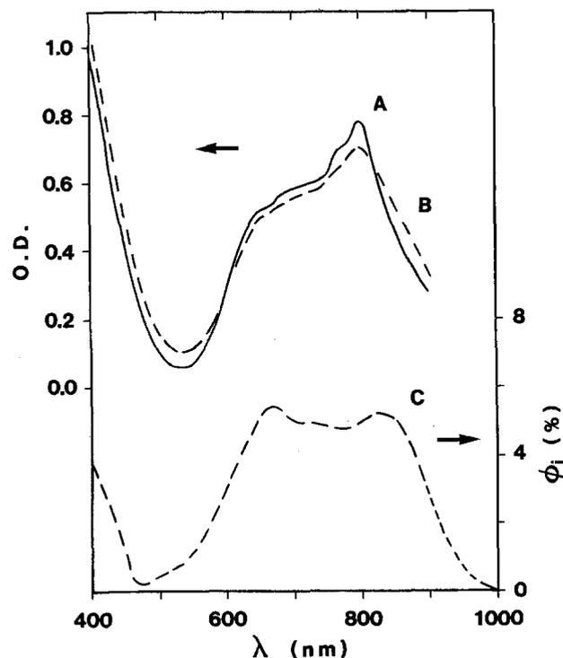
Fig. 5. Absorption spectra (curves A and B) and incident quantum efficiencies,  $\phi_i$  (curve C) of a  $0.16 \mu\text{m}$  thick CIAIPc film slowly grown on hot  $\text{SnO}_2$  before (A) and after transformation I (B and C).
