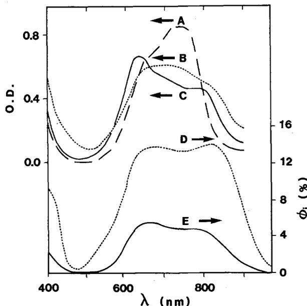
Fig. 1. Absorption spectra (curves A, B, and C) and incident quantum efficiencies  $\phi_1$  (curves D and E) of a 0.16  $\mu\text{m}$  and  $\sim 0.6 \mu\text{m}$  thick ClAlPc film, respectively; before (A), after transformation I (B, D), and after transformation H (C, E).
