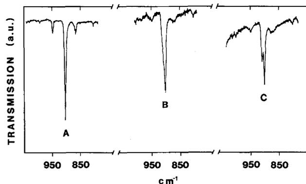
Fig. 13. Evolution of the 900  $\text{cm}^{-1}$  infrared band before transformation (A), after transformation I (B), and after transformation H (C) of a ClAlPc film.
