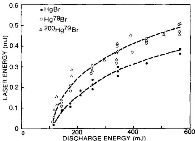
FIG. 1. Electric discharge laser performance for three isotopic compositions.
