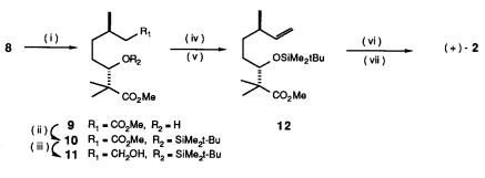
(i) K<sub>2</sub>CO<sub>3</sub>, MeOH (90%) (ii) t-BuMe<sub>2</sub>SiOSO<sub>2</sub>CF<sub>3</sub>, 2,6-lutidine, CH<sub>2</sub>Cl<sub>2</sub> (98%) (iii) LiAlH<sub>4</sub>, Et<sub>2</sub>O, -78°C (85%) (iv) o-O<sub>2</sub>NC<sub>6</sub>H<sub>4</sub>SeCN, n-Bu<sub>3</sub>P, THF (v) H<sub>2</sub>O<sub>2</sub> (91%) (vi) RuCl<sub>3</sub>, NaЮ<sub>4</sub>, CH<sub>3</sub>CN-CCl<sub>4</sub>-H<sub>2</sub>O (1:1:2) (vii) 5% HF, CH<sub>3</sub>CN (79% from **12**)
