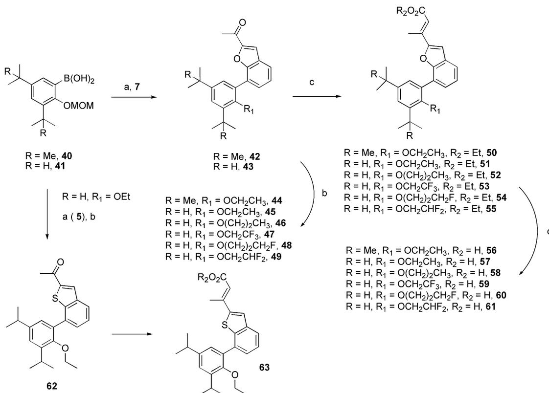
**Scheme 3.** 2,7-Disubstituted 1-benzofuran and 1-benzothiophene RXR modulators synthetic scheme. Reagents: (a) Pd(PPh<sub>3</sub>)<sub>4</sub>, **6** or **7**, toluene/EtOH, 2M Na<sub>2</sub>CO<sub>3</sub>, reflux. (b) R-Br, Cs<sub>2</sub>CO<sub>3</sub>, DMF, rt. Steps (c) and (d) identical of these described in Scheme 2 (b,c).
