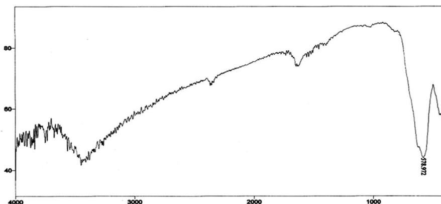
**Fig. 2** FTIR spectrum of nano- $\text{Fe}_3\text{O}_4$
