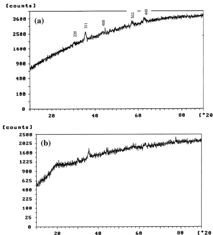
**Fig. 8** X-ray diffraction pattern of the nano-Fe<sub>3</sub>O<sub>4</sub> (a) and nanocomposite (b)
