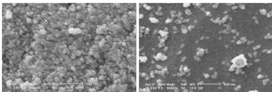
**Fig. 1** SEM images of nano- $\text{Fe}_3\text{O}_4$
