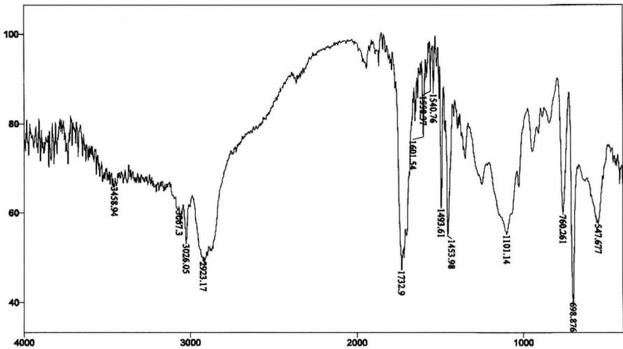
Fig. 5 FTIR spectrum of nano-Fe<sub>3</sub>O<sub>4</sub>-PS-Co-[PAA-g-PEG]
