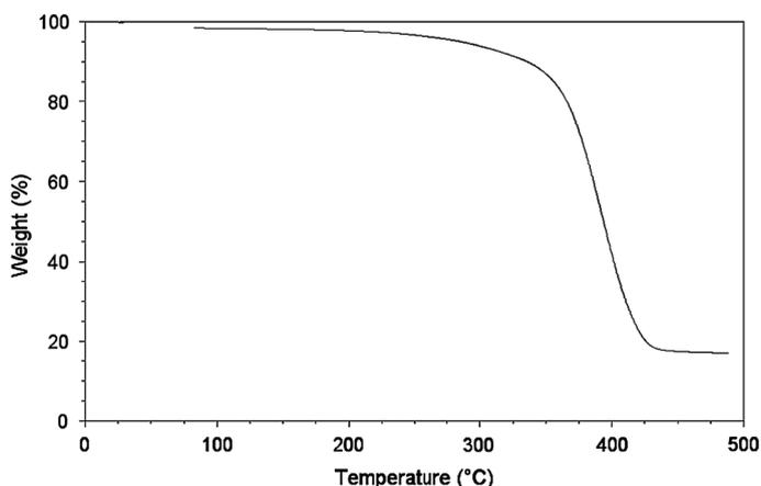
**Fig. 6** TGA diagram of nano-Fe<sub>3</sub>O<sub>4</sub>-PS-Co-[PAA-g-PEG]
