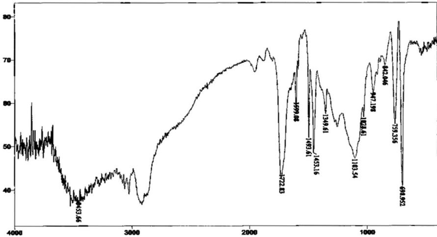
Fig. 4 FTIR spectrum of copoly[(styrene/acrylic acid)/grafted PEG]
