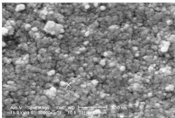
**Fig. 7** SEM images of nano-Fe<sub>3</sub>O<sub>4</sub>-PS-Co-[PAA-g-PEG]
