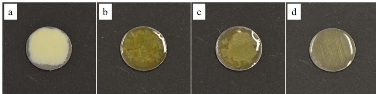
**FIGURE 4** Polymer films cast from molten mixtures: (a) **M1/F1**, (b) **M2/F2**, (c) **M3/F3**, and (d) **M4/F4**. [Color figure can be viewed in the online issue, which is available at [wileyonlinelibrary.com](http://wileyonlinelibrary.com).]
