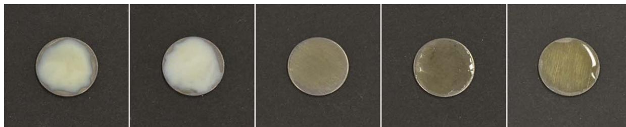
**FIGURE 11** Polymer films cast from molten mixtures of **M4/F4** and **M1/F1** in ratios of (a) 0:100; (b) 20:80; (c) 50:50; (d) 80:20; and (e) 100:0. [Color figure can be viewed in the online issue, which is available at [wileyonlinelibrary.com](http://wileyonlinelibrary.com).]
