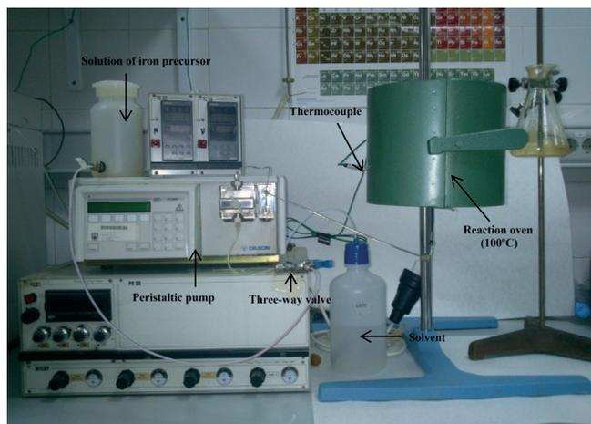
**Figure 8.** Experimental setup for the continuous flow preparation of Fe/AlZn-SBA materials.
