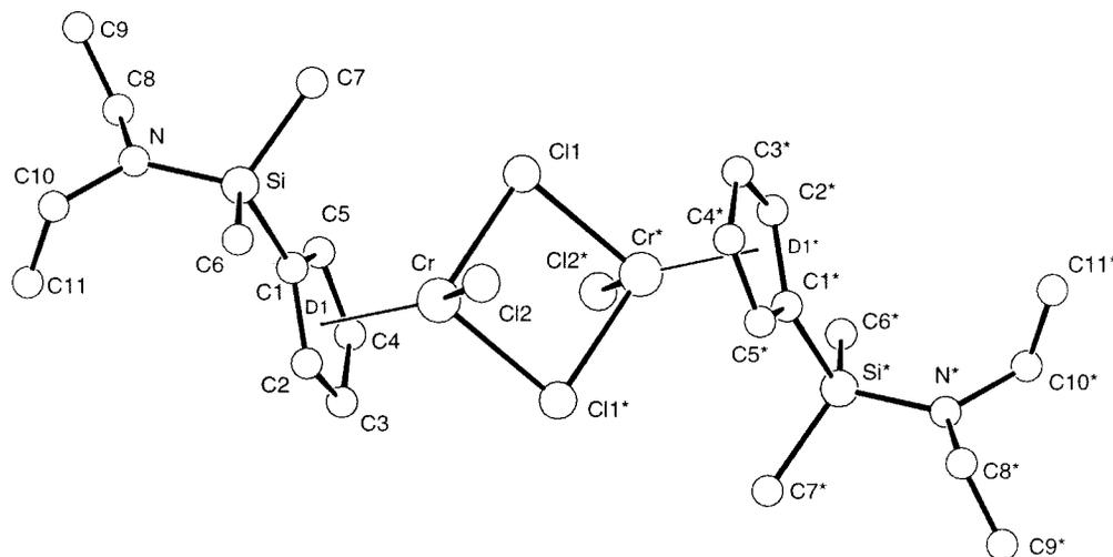
**Figure 3.** Molecular structure of  $[(\text{Et}_2\text{NSiMe}_2\text{C}_5\text{H}_4)\text{CrCl}_2]_2$  (**27**). Selected bond distances (Å) and angles (deg) are as follows: Cr–D1 = 1.862, Cr–Cl1 = 2.365(1), Cr–Cl1\* = 2.375(1), Cr–Cl2 = 2.268, Cr–Cr\* = 3.352(1); D1–Cr–Cl1 = 121.3, D1–Cr–Cl2 = 126.3, Cl1–Cr–Cl1\* = 91.4, Cl1–Cr–Cl2 = 95.1(1)°.
