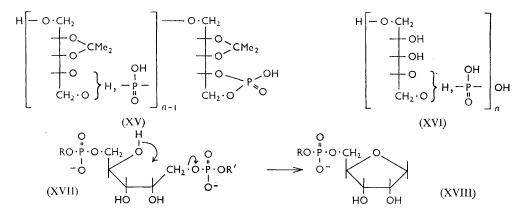
(XV). Hydrolysis with dilute acid removed the isopropylidene groups and opened the terminal cyclic phosphate group to give the polymer (XVI), which was purified by dialysis and isolated as its lithium salt.
