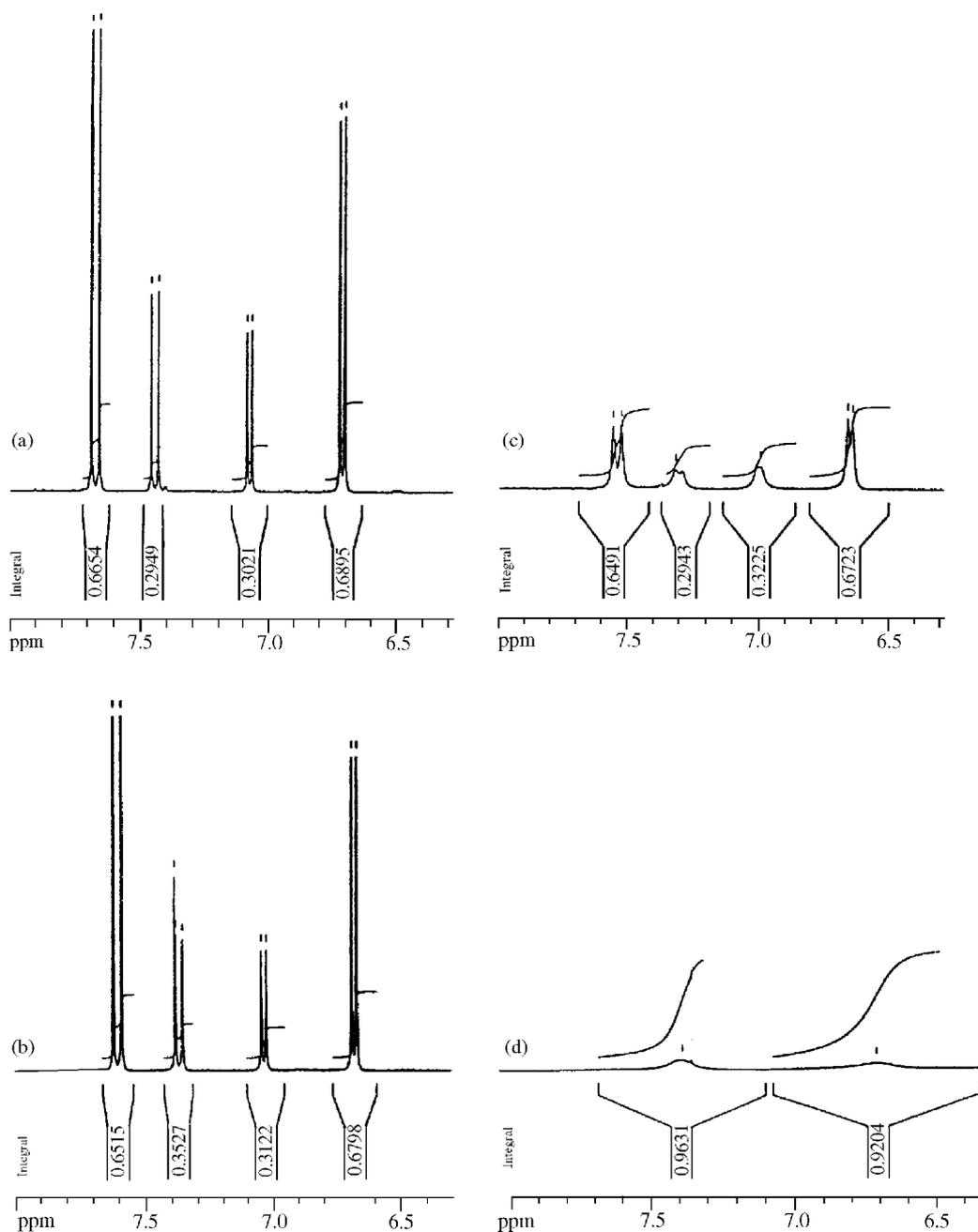
Fig. 2.  $^1\text{H}$  NMR spectra of **2** in  $(\text{CD}_3)_2\text{CO}$  recorded at  $-4\text{ }^\circ\text{C}$  (a);  $-20\text{ }^\circ\text{C}$  (b);  $0\text{ }^\circ\text{C}$  (c) and  $20\text{ }^\circ\text{C}$  (d).
